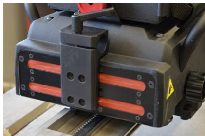
Silicone covers protect against dirt and spatter
