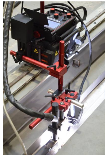
Seam tracking works with and without oscillation
