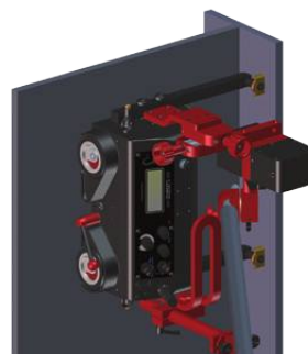
Fillet Welding with oscillator
