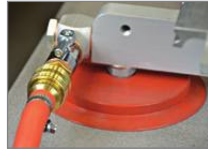
Cut-off valve (for entry vacuum unit) ZWR-0541-10-01-30-0
